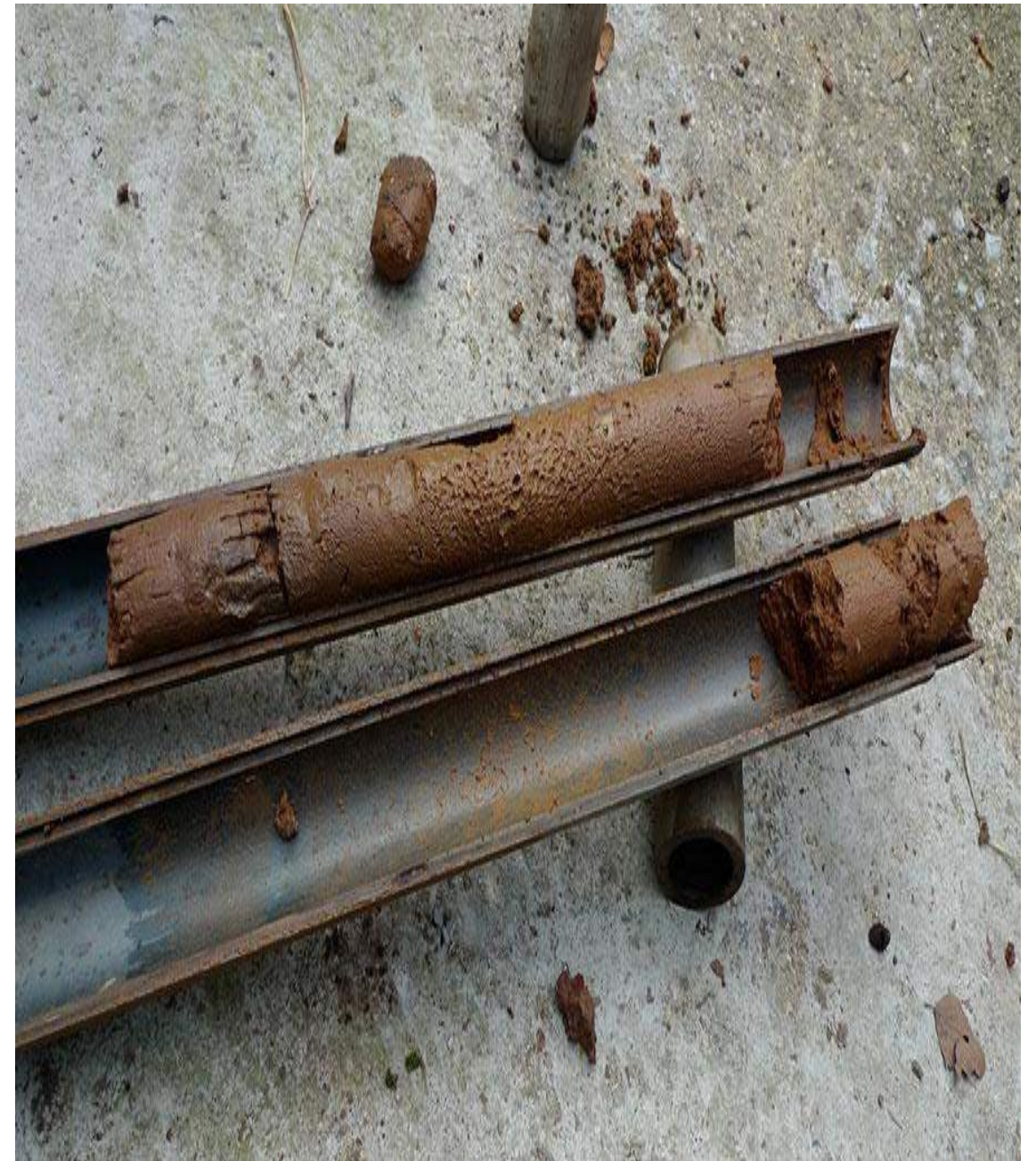
Figure 14.12 Standard split spoon sampler: (a) Schematic diagram and (b) typical sampler.
